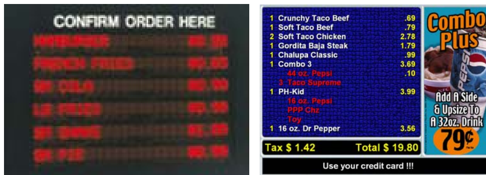
Figure 1 - LED vs. LCD OCS Screens
