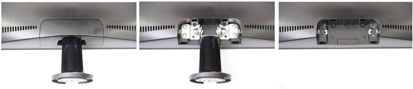
Figure 5 - Remove Stand from Monitor
