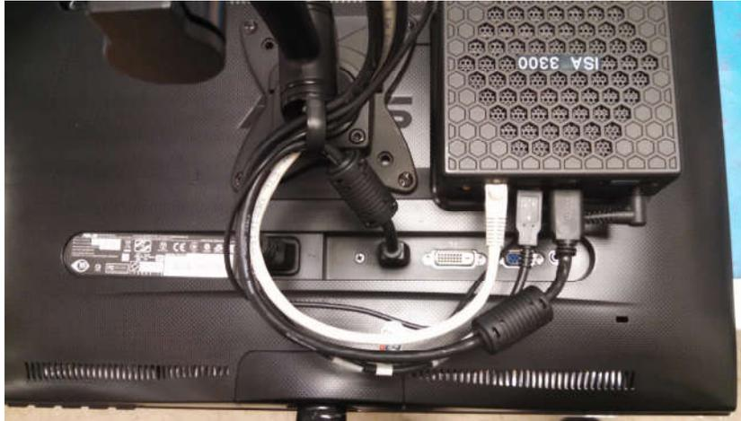
Figure 8 – Mounted Controller and Cable Connections
