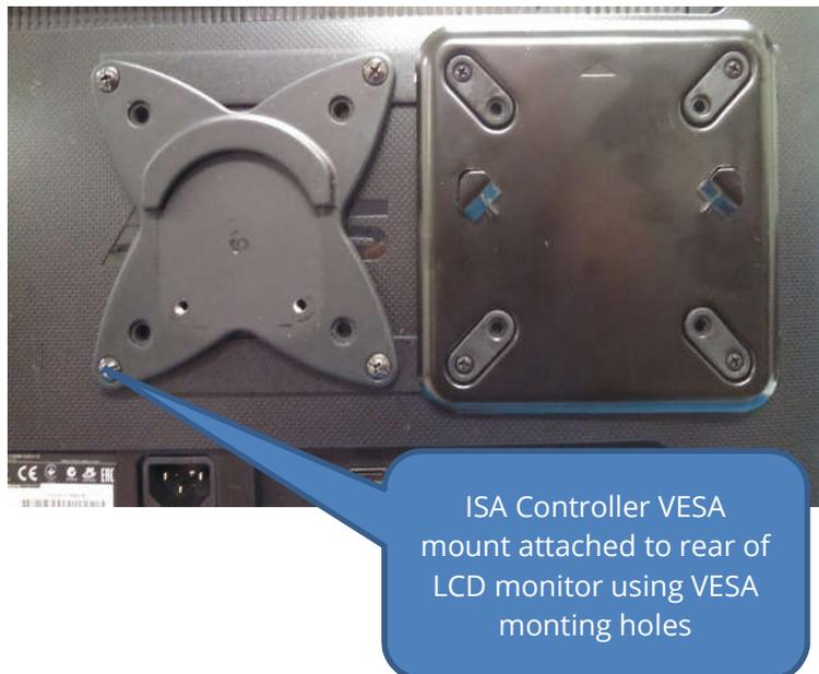
**Figure 7: Attach Controller Mounting Bracket assembly to rear of LCD monitor**
