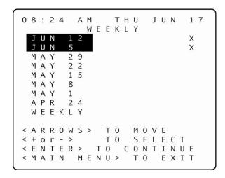
**NOTE:** The days shown on the screen are the first days of the most current seven business weeks as programmed in Set Parameters for a specific Timer.
