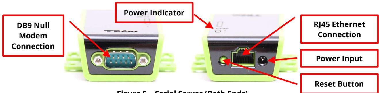
Figure 5 – Serial Server (Both Ends)
