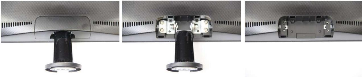
**Figure 8 - Remove Stand from Monitor**
